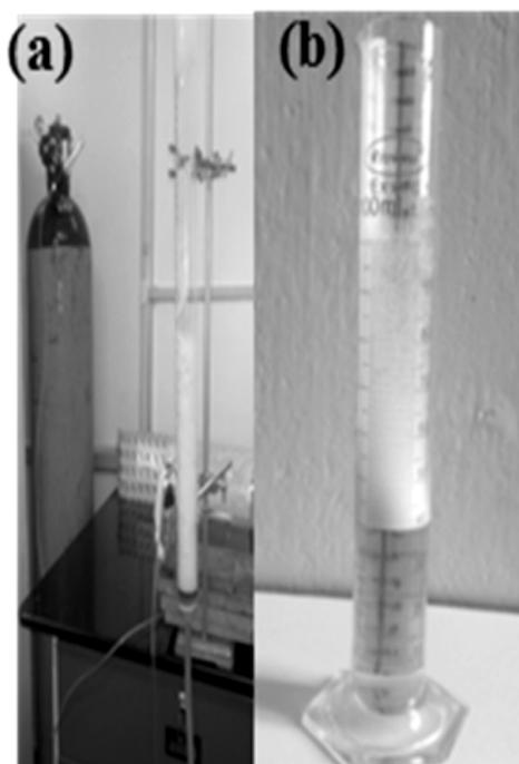
Fig. 2. Experimental set-up for Foaming Ability and Stability by (a) Bickerman's Method and (b) Shaking Tube Method.
