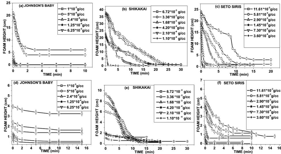
Fig. 5. Foam height against time by (a), (b), (c) Bikerman's Method and (d), (e), (f) by Shaking Tube Method.
