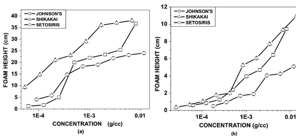
Fig. 4. Variation of Foam Height with concentration by (a) Bikerman's Method. (b) Shaking Tube Method.
