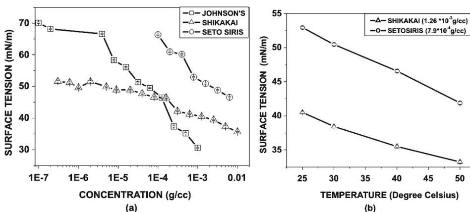
Fig. 3. (a) Variation of surface tension with concentration for different surfactants (at  $25 \pm 2^\circ\text{C}$ ). (b) Effect of temperature on surface tension of natural detergents.
