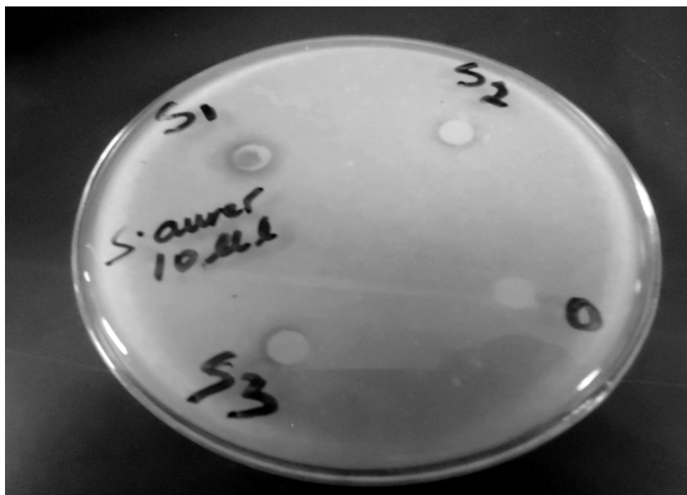
Fig. 11. Zones of inhibition by 10 \mu l of 5 mg/ml suspension of silver nanoparticles synthesized using different plant leaf extracts as reductant and stabilizers against Staphylococcus aureus ; S 1 = sun flower ( helianthus annuus ) mediated Ag nanoparticles; S 2 = Castore Oil ( Ricinus Communes ) mediated Ag nanoparticles; S 3 = Khat ( Catha Edulis ) mediated Ag nanoparticles; O = Control (Distilled Water).
